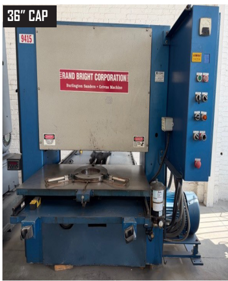
Burlington Rand Model S36X75R, 36" Abrasive Belt Grinder.
