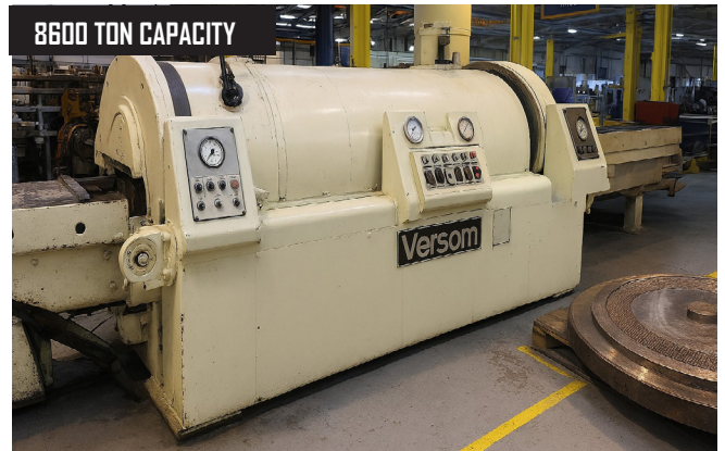
Versom Wheelon Model 8600R-36-92 Direct-Acting Hydraulic Forming Press, 8600 Ton Capacity, 5000 psi Forming Pressure, 36" x 92" Tray Size.
