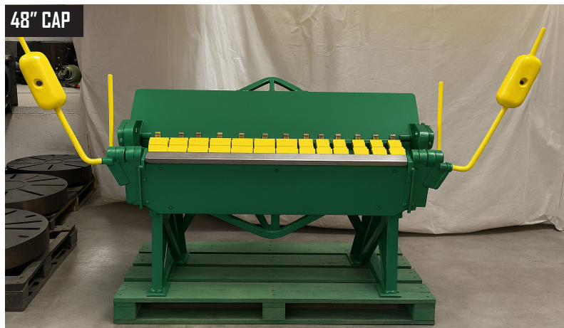
48" CAP Chicago Model L31 Box and Pan Hand Brake, 48" x 14 Gauge Capacity.
