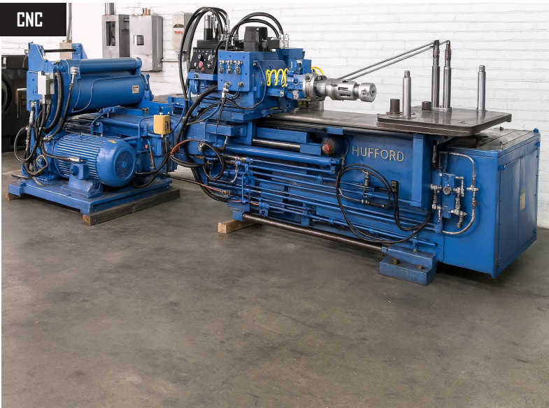
L & F Hufford Model A-5 CNC Stretch Wrap Forming Machine, 12 Tons, 115" Distance Between Jaws, 20" Tension Cylinder Stroke, 30" Tension Cylinder Swing, w/ DeMott CNC Controls and Remote Hand Controls.
