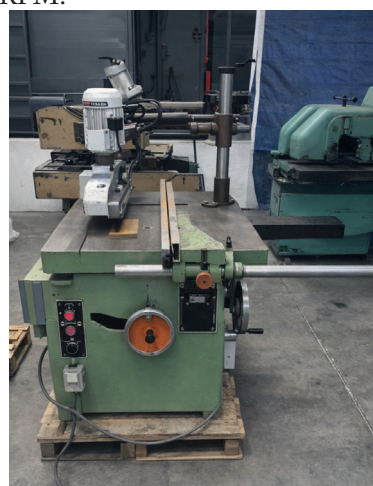
Poloni 16" Tilting Arbor Table Panel Saw w/ Holzher 1112 Power Feeder.
