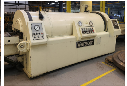
Versom Wheelon Model 8600R-36-92 Direct-Acting Hydraulic Forming Press, 8600 Ton Capacity, 5000 psi Forming Pressure, 36" x 92" Tray Size.
