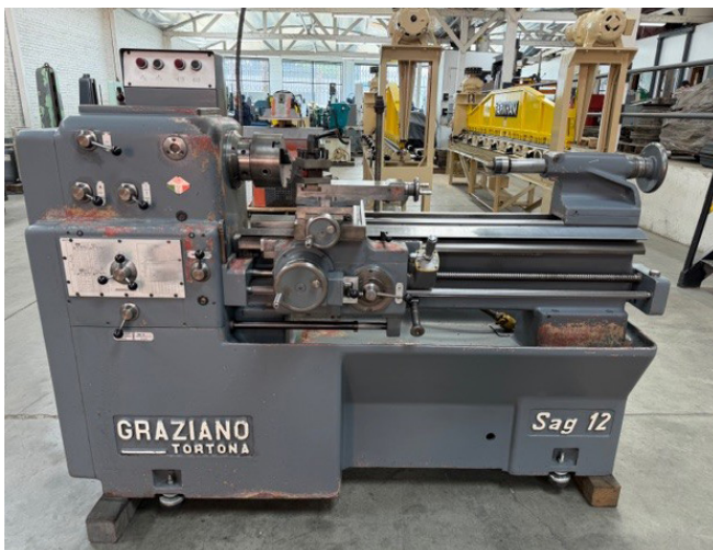
Graziano-SAG 12.5" x 40" Engine Lathe, English-Metric, 3 and 4 Jaw Chuck, 7-2000 RPM.
