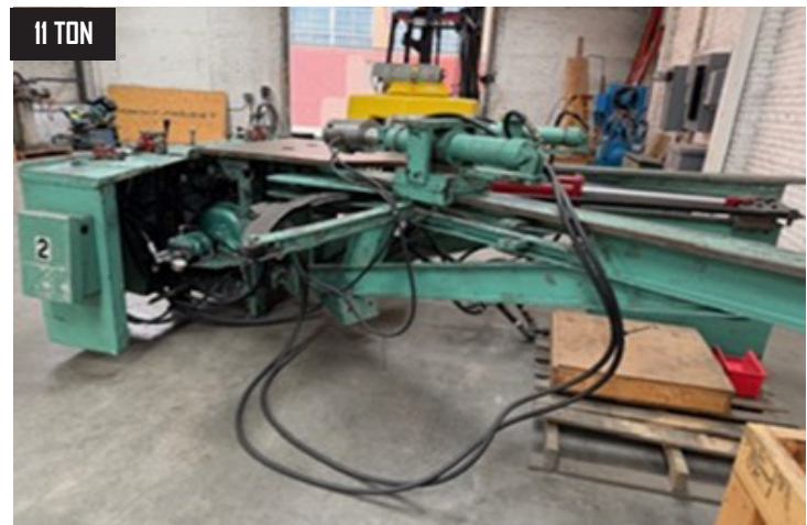
11 TON NAS Division 11 Ton Stretch Wrap Forming Press w/ 136" Max Length of Tension Cylinders fully retracted, Equipped w/ 1 set of 3" jaws and Gripper jaws.
