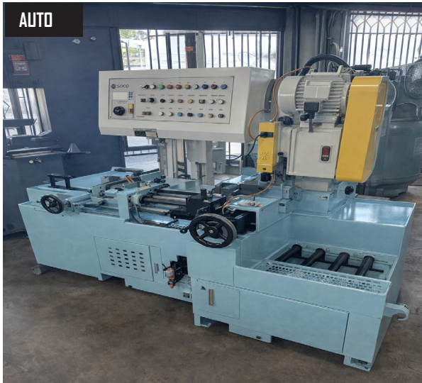
AUTO 2004 Soco HVS-375-FA-DR Programmable Automatic Cold Saw, 14.76" Blade, 4.5" Bar Capacity.
