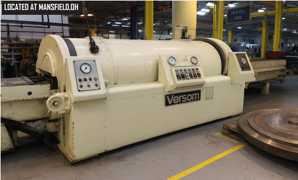
Versom Wheelon Model 8600R-36-92 Direct-Acting Hydraulic Forming Press, 8600 Ton Capacity, 5000 psi Forming Pressure, 36" x 92" Tray Size.
