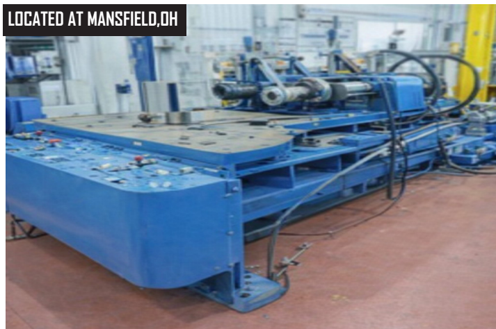
Hufford Model A-10 Stretch Wrap Forming Press, 17.5 Ton Forming, 219" Distance Between Jaws, Hydraulic Clamping, Simultaneous Arm Motion Swing, s/n BHW-P-361.
