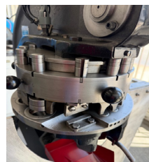
Rotex Model 18AK, 8 Ton Turret Punch, s/n 14119
