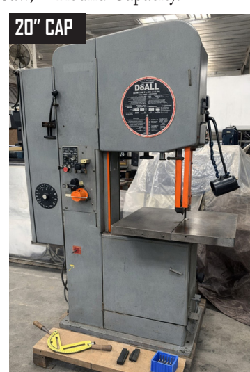
20" CAP Do All Model 2013-20, 20" Vertical Band Saw w/ Welder.
