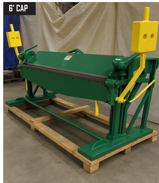
6' CAP Roper Whitney Jensen Model 616 Leaf Hand Brake, 6 Ft x 16 Gauge Capacity.
