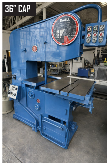
36" CAP Do All Model 3612-3, 36" Vertical Band Saw, 3 Speed Gear Box, Power Feed Table, 25-6000 RPM.
