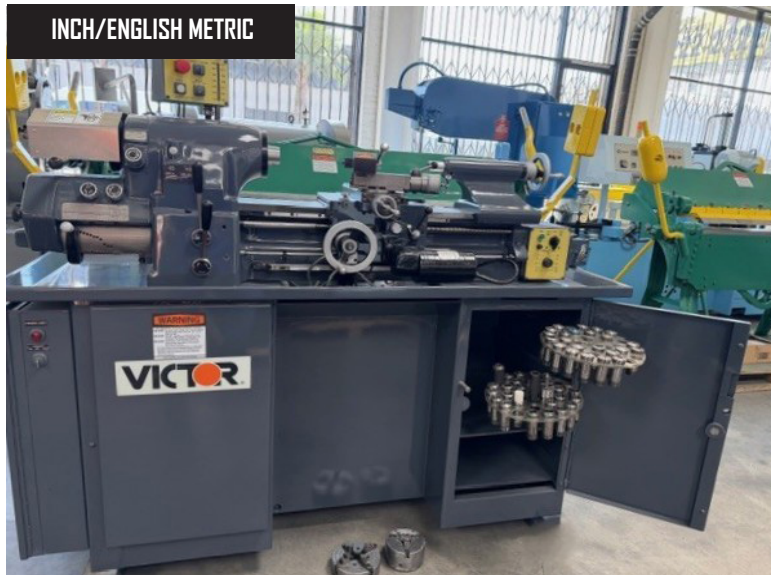
Victor Model 518EM Tool Room Lathe w/ English Metric Tool Room Lathe, 11" x 18" Capacity, DRO and 5C Collets, s/n 21093.
