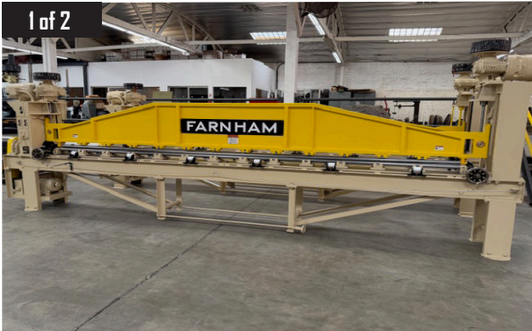
Farnham Model 1510-E, 15 Ft Capacity Forming Rolls, 1.625" Top and Bottom Rolls, s/n 3-43-11.
