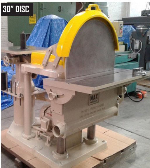
Max 30" Combination Disc 30DVS and Spindle Sander VS-1, 15" F-B Working Surface x 38.5" L-R For Disc Sander and 24" x 24" Spindle Sander Table.
