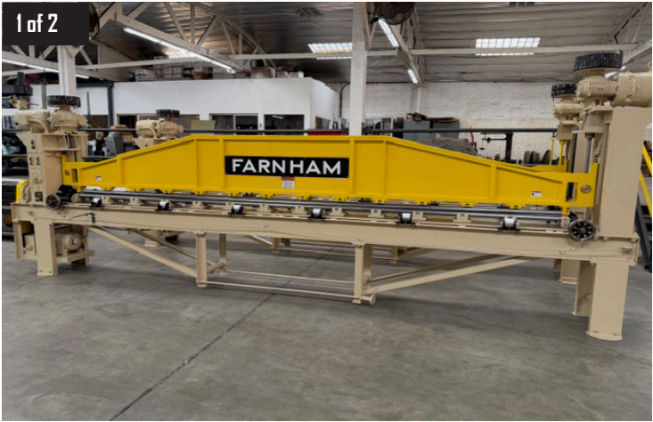
1 of 2 Farnham Model 1510-E, 15 Ft Capacity Forming Rolls, 1.625" Top and Bottom Rolls, s/n 3-43-11.
