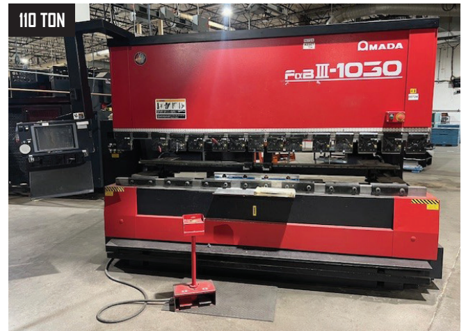
2001 Amada FDB-1030NT, 118.1" x 110 Ton CNC Hydraulic Press Brake, 7 Axis Amada AMNC/PC Controls, s/n 10300119.
