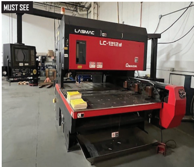
1994 Amada Model LC1212Alpha CNC Laser Cutting Machine, CO2, 1.5 KW Laser Capacity, w/ Fanuc 16-L Controls, 4' x 8' Sheet Capacity, 0.5" Maximum Cutting Capacity, s/n 12120057.
