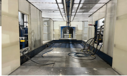
Nordson Electrostatic Powder Coating Booth Model Horizon 400 w/ Manual Guns and Controls.
