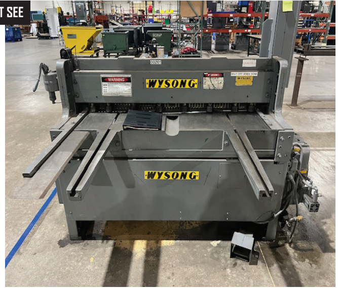
Wysong 52" Power Mechanical Shear w/ Squaring Arm and Foot Pedal.
