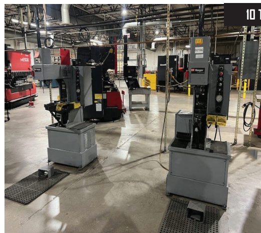
10 TOTAL 2 of 10) Haeger HP6-C, 6 Ton Hydraulic Hardware Insertion Press w/ Bowl Feed.
