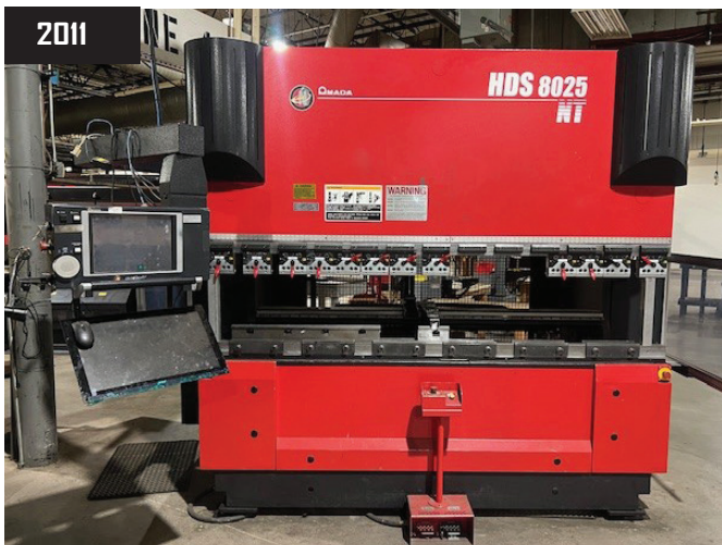
2011 Amada HDS-8025NT 102.4" x 88 Ton Servo-Hydraulic Press Brake, w/ AMNC-PC 5 Axis Control, s/n 82504198.
