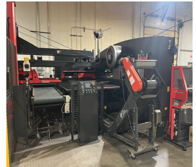
2011 Amada EMLK 3610 NT CNC Hybrid Servo-Electric Laser/Punch Combination Machine, 33 Ton Capacity, 4.0 KW Laser, 58 Station Thick Turret, 4 Auto Index, 60" x 100 Laser Cutting and 60" x 120" Punching Sheet Size, Brush Table, Amada AMNC PC Controls, and Amada AASR 510M Automation Tower, s/n 43612064.
