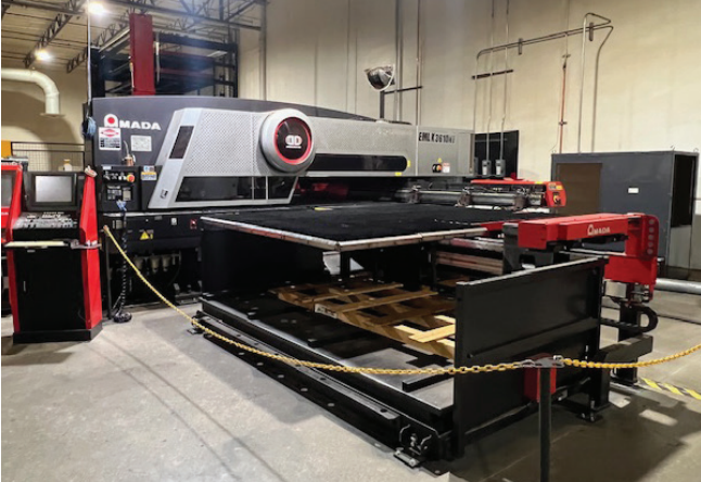
2011 Amada EMLK 3610 NT CNC Hybrid Servo-Electric Laser/Punch Combination Machine, 33 Ton Capacity, 4.0 KW Laser, 58 Station Thick Turret, 4 Auto Index, 60" x 100 Laser Cutting and 60" x 120" Punching Sheet Size, Brush Table, Amada AMNC PC Controls, and Amada AASR 510M Automation Tower, s/n 43612064.
