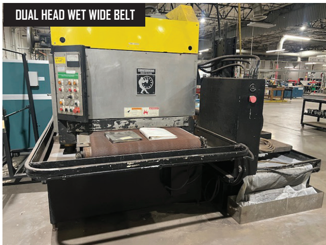
Timesaver 137-2 HD CMW 37" Dual Head Wet Wide Belt Sander w/ Controls and Filtration System, s/n 22561.
