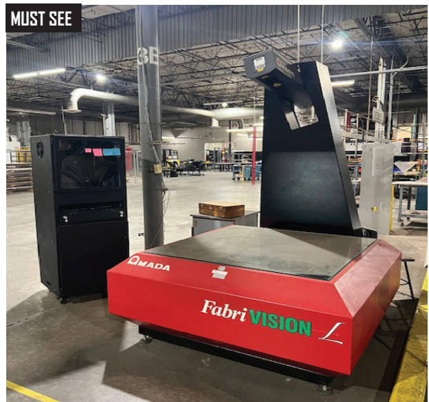
Amada-Virtek LPS-1E Laser Scanning Inspection System, s/n 11027917.
