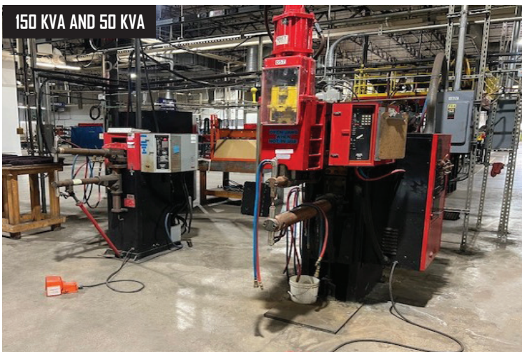
150 KVA AND 50 KVA Janda 150 KVA and Janda 50 KVA Spot Welders with iii CNC Controls.
