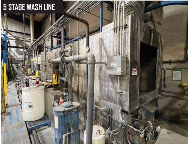
GFC General Fabrication Corporation 5 Stage Stainless Steel Wash Line For Powder Coating.
