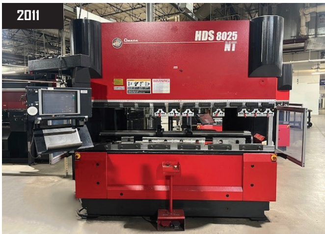
2011 Amada HDS-8025NT 102.4" x 88 Ton Servo-Hydraulic Press Brake, w/ AMNC-PC 5 Axis Control, s/n 82504216.
