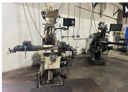
Acer Vertical Mill w/ Variable Speed, DRO and Power Feed & Bridgeport CNC Ez Trak Milling Machine.
