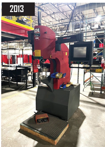
2013 2013 Haeger 824WT-4H, 8-ton Hydraulic Hardware Insertion Press w/ Bowl Feed, 24" Throat Depth, Window Touch 4e Controls.
