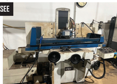
Kent Hydraulic Surface Grinder, Automatic, Controls and Filtration System.
