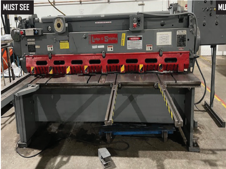
Lodge & Shipley Model 0208 8' x 10 GA Power Shear, Sq Arm, Front Operated Power Back Gage.
