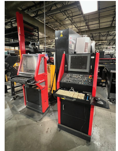
2008 Amada EMLK 3610 NT CNC Hybrid Servo-Electric Laser/Punch Combination Machine, 33 Ton Capacity, 4.0 KW Laser, 58 Station Thick Turret, 4 Auto Index, 60" x 100 Laser Cutting and 60" x 120" Punching Sheet Size, Brush Table, Amada AMNC PC Controls, and Amada AASR 510M Automation Tower, s/n 43012034.
