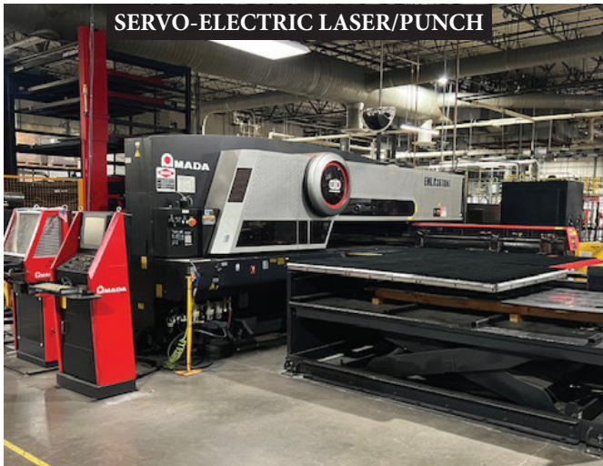
2008 Amada EMLK 3610 NT CNC Hybrid Servo-Electric Laser/Punch Combination Machine, 33 Ton Capacity, 4.0 KW Laser, 58 Station Thick Turret, 4 Auto Index, 60" x 100 Laser Cutting and 60" x 120" Punching Sheet Size, Brush Table, Amada AMNC PC Controls, and Amada AASR 510M Automation Tower, s/n 43012034.
