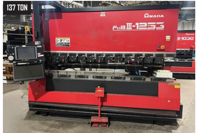
2000 Amada FDB-1253NT, 118.1" x 137 Ton CNC Hydraulic Up-acting Press Brake, Multi Axis Amada AMNC/PC Controls, s/n 12530259
