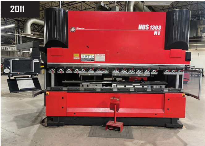
2011 Amada HDS-1303NT 126.8" x 1143 Ton Servo-Hydraulic Press Brake, Multi Axis AMNC-PC Controls, 87" Distance Between Frames, s/n 13304265.
