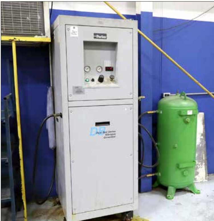
Parker DB-5 PSA Dual Bed Series Nitrogen Generator with Parker Surge Tank
