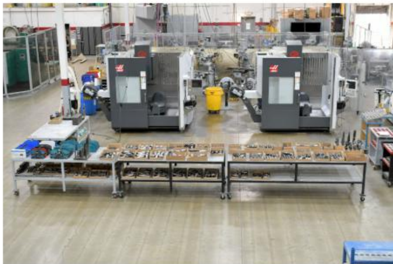
(2) 2017 Haas UMC 750, 5-Axis Universal CNC Machining Centers
