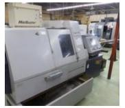
Citizen M20 CNC Swiss Type Automatic Screw Machine with Cincom CNC Control, Mist Collector, and Spego Turnamic Barfeed
