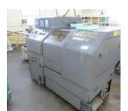
Hardinge Conquest **CS-GT Gang Style** CNC Lathe, Parts Chute, Mini Rhino **Bar Barfeed**
