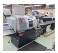
Citizen C16 Type VI **CNC Swiss Screw** Machine with Citizen CAV16C-IS Magazine Barfeeder, Long Parts Attachment
