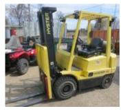
Hyster 40 Forklift W 42" Forks, Triple Mast, Side Shift and Fork Tilt
