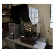
Nikon 6C Optical Comparator, 11" Screen, 5" x 9" Stage, Surface and Profile Illumination, **Micrometer Table** Feeds
