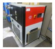
Keltech Technolab Model KRAD-200 Air Dryer
