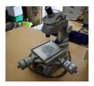
Mitutoyo Toolmakers Microscope, 15X Eyepiece Lens, .0001"Travel Indicators
