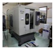
Brother TC-311 **CNC** Vertical Machining Center, (2) Pallet Changer, 10 Station ATC,
